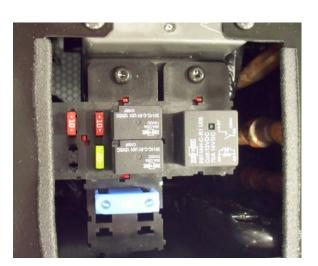
**R3.** This relay controls the voltage to the compressor.
