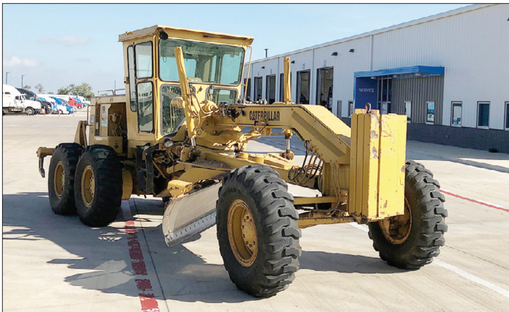
Texas Truck A/C installed a complete Red Dot aftermarket A/C system on this Caterpillar 12G motor grader, which is powered by a CAT 3306 engine.
